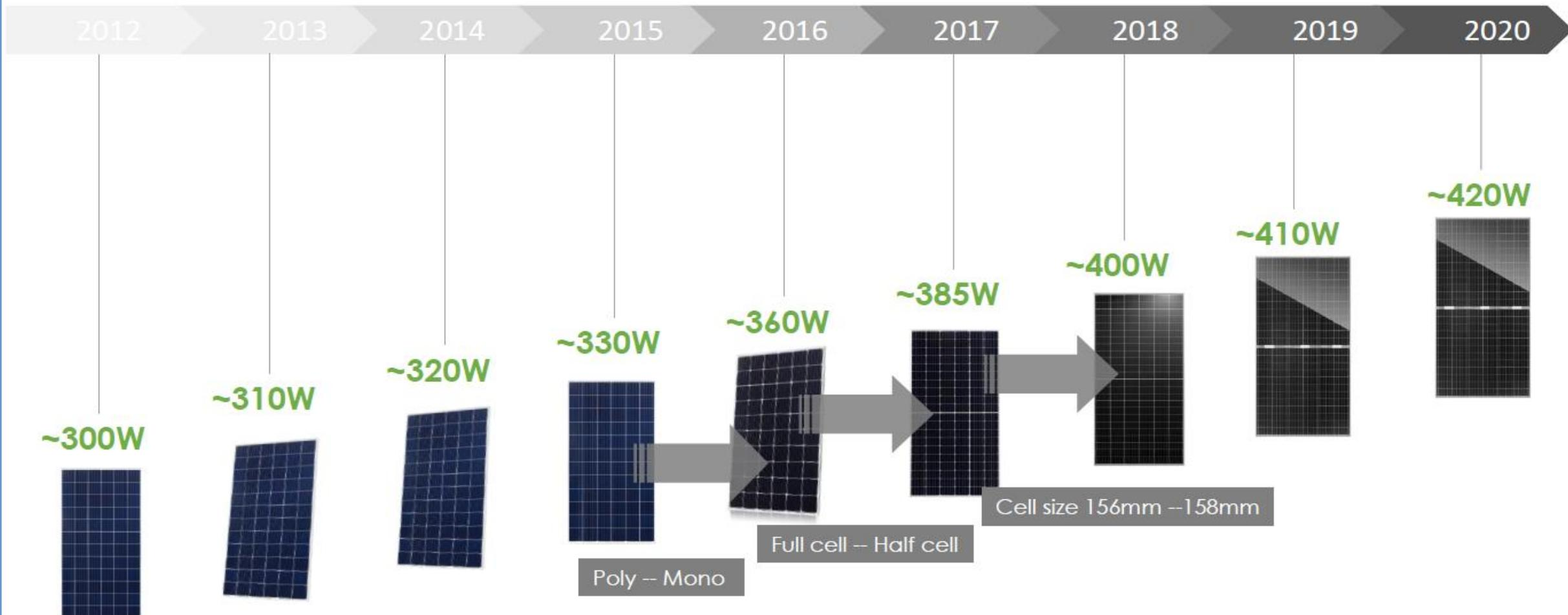
Mass-produced module power output has been increasing continuously, 10 W annually on average.
